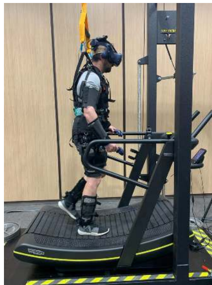
Figure 1. Passive treadmill with fall-restraint system.
